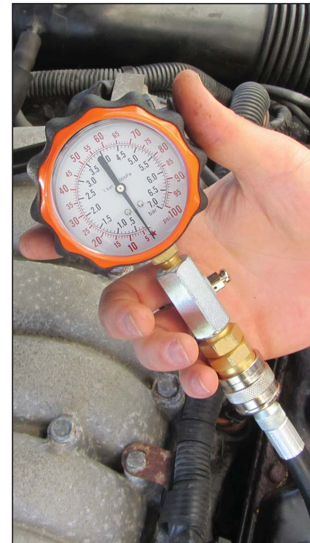
74427: Gauge Assembly on the TU-30A
